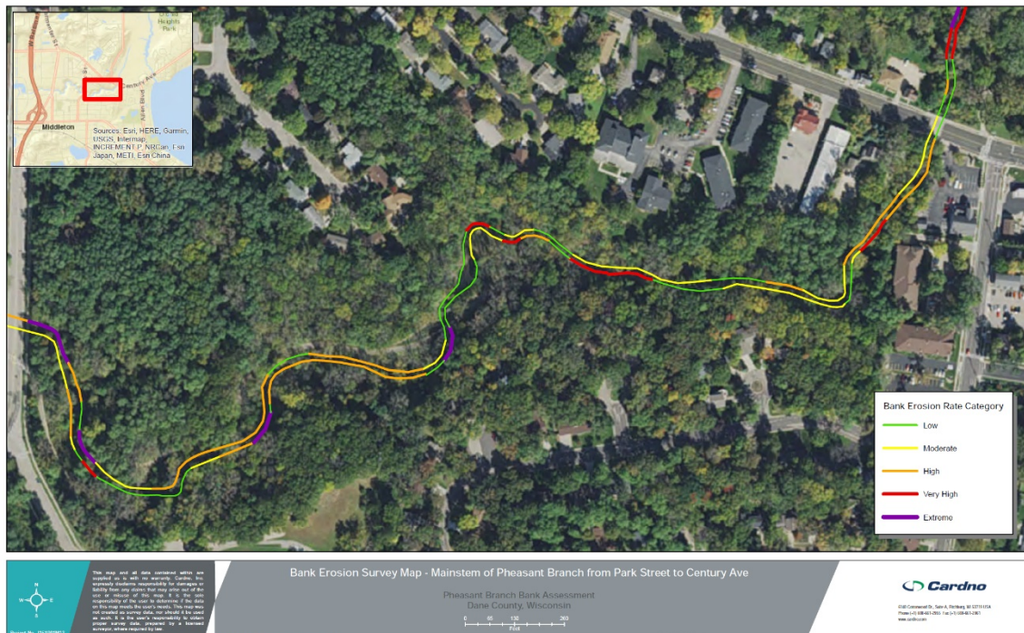
Figure 61: Location of streambank restoration areas identified between Park Street and Century Avenue
