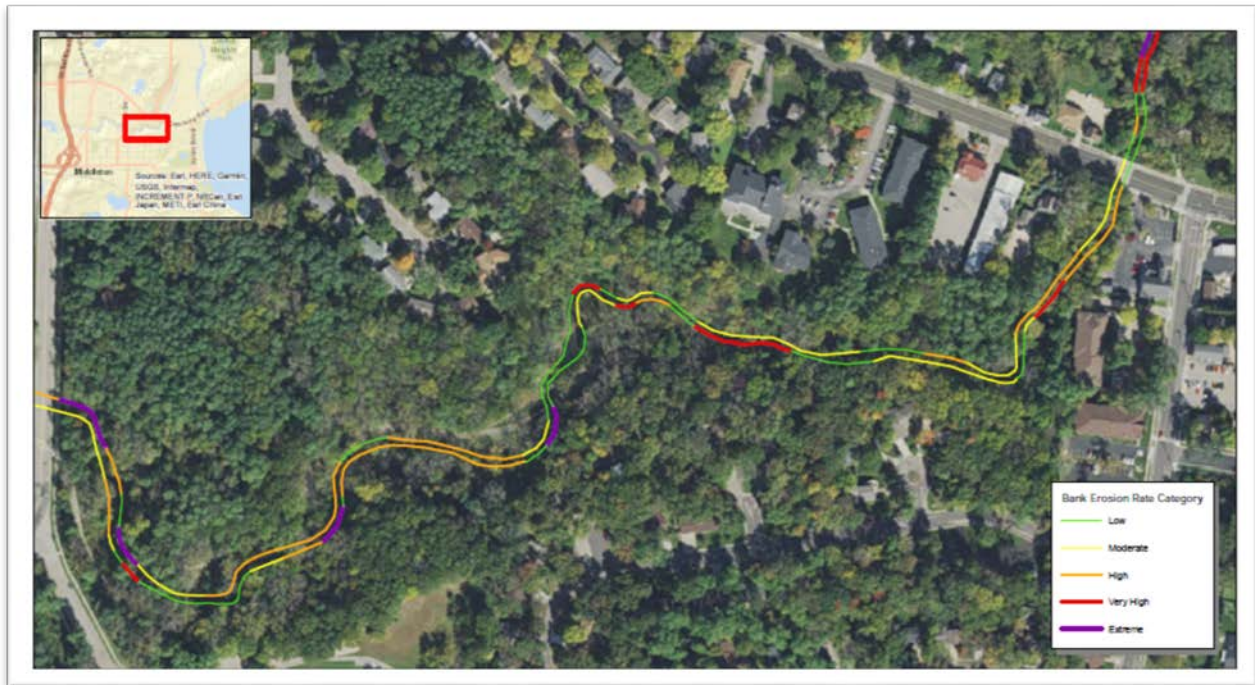
Figure 9: BEHI model streambank erosion risk assessment for mainstem of Pheasant Branch between Park Street and Century Avenue
